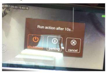
When the vehicle ignition switch (ACC) is turned off or a car charger is unplugged, the device will automatically display "shutdown", "parking" and "cancel" menu option as shown in the picture above. When you select "parking" option, it will be entered into parking monitor mode.
