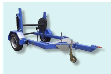
Trailer fit to transport and unwind reels of cable weighting up to 8000 kg.
