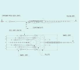
**Balanced type** running board for 6-bundle conductors fit for connecting the pulling rope to 6 conductors.
