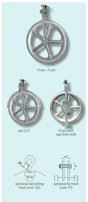
Single sheave running out block fit for stringing one conductor. Aluminium sheave mounted on sealed ball bearings. Groove lined with nylon sectors. Openable galvanised steel frame with non-fleeting device. Standard swivelling fork attachment.
