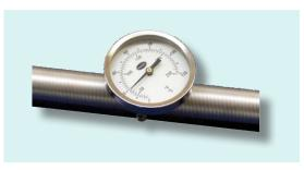
Thermometer for conductors. The dial diameter 80 mm, with incorporated sensor, can be fixed easily on the conductor by means of its elastic clamp. Double scale (°C and °F).
