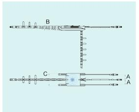
**F153.2 Balanced type** running board for 2-bundle conductors, fit for connecting the pulling rope to 2 conductors.
