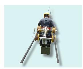
Bicycle for single, twin, 3- and 4-bundle conductor lines.
