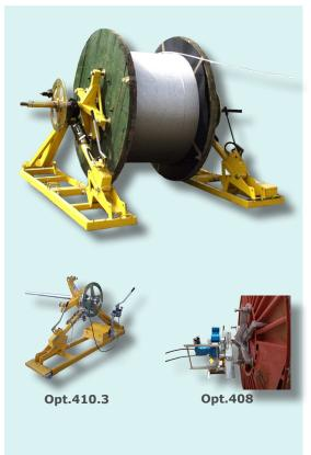
Stands fit for steel or wooden reels, used for lifting a reel and braking it while stringing the conductor/cable. The reel stands, as an option, can be hydraulically driven by a hydraulic power unit. Reel-stands are supplied in pairs.
