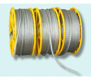
Anti-twisting galvanised steel rope specifically designed for stringing operations. Made up of 12 braided strands. High resistant to break, antitwisting, flexible, safe and easy to handle. The linear contact between the braided strands grants a low stress on the rope. Supplied wound up on steel or wooden reels.
