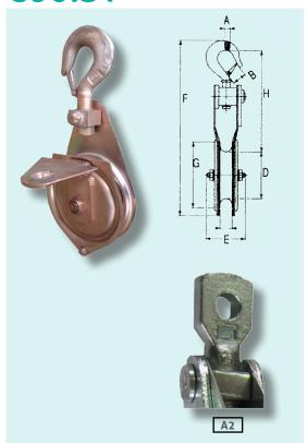
Openable snatch block. Galvanised steel sheave mounted on ball bearings. Galvanised steel frame with openable side. Standard hook attachment.
