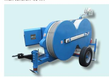
Hydraulic tensioner fit to string one or two conductors or optical fiber cables. One hydraulic circuit allows to tension at constant force even varying the speed of stringing. Equipped with engine for pull-back performances.
