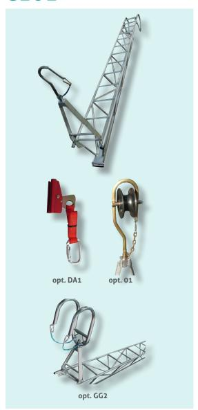
Anchoring ladder made of light aluminum alloy, with steps made of antislipping material and suspension hooks in hot-dip galvanized steel. The ladder is complete with a fix hook for tower, 220mm opening, and a swivel hook for leaning on the conductor, to use the ladder in horizontal position. The ladders have trapezoidal shape.
