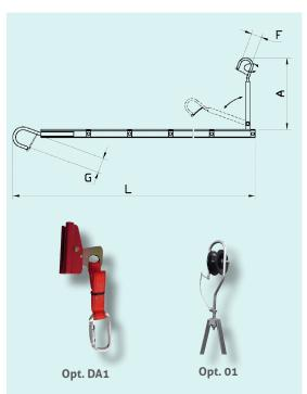
Suspension ladder fit for vertical or horizontal use.
