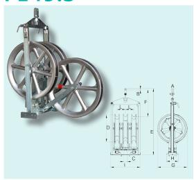
Detachable three-sheave running out block fit for stringing two- three-bundled conductors. The frame contains 3 running-out blocks that can be used singularly. Aluminium sheaves mounted on sealed ball bearings. Grooves lined with nylon sectors. Galvanised steel frame. Central sheave mounted on double bearings. Demountable attachment revolving by 90°.
