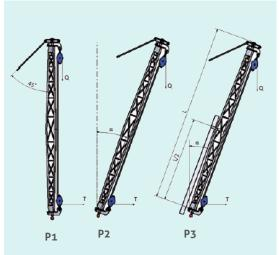
Gin poles made of aluminium alloy tubular structure welded with TIG system. Made of two or more separated sections.
