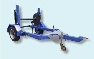
Trailer fit to transport and unwind reels of cable weighting up to  $4000 \ \text{kg}$ .
