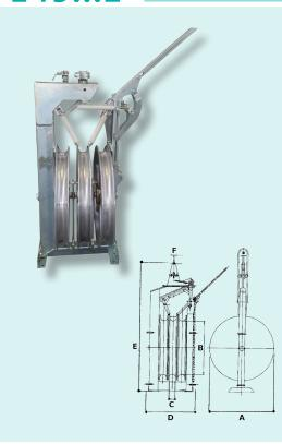
Three-sheave block fit for stringing a pilot rope by helicopter. Proper devices allow to position the pulling rope in the sheave groove, and keep it inside the groove during stringing operations. Aluminium sheave mounted on waterproof bearings. Groove lined with nylon sectors. Galvanized steel frame. Fix attachment.
