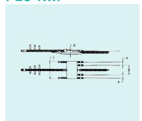
**Fixed type** running board for 4-bundle conductors fit for connecting the pulling rope to 4 conductors. The running board is made up of:
