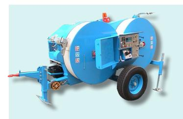
Hydraulic tensioner fit to string one conductor or fiber optic cable. One hydraulic circuit allows to tension at constant force even varying the speed of stringing. Equipped with engine for pull-back performances.
