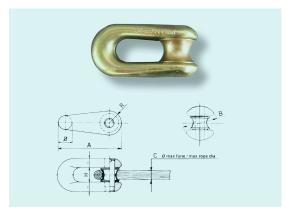
Joint made of high tensile galvanised steel, fit to connect pilot rope lenghts and pulling rope. Designed to pass on the capstan grooves of pullers or puller/tensioners.
