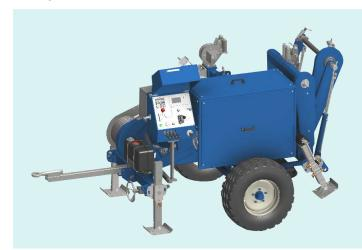
Hydraulic puller fit to pull one rope in stringing operations of overhead transmission lines. One hydraulic circuit allows to continuously vary the speed in both directions by operating one control device.
