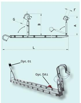
Suspension ladder fit for vertical and horizontal use.
