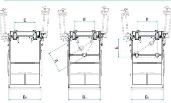
note:the dimensions E are adjustable 400-457-500-600 mm. Line cars with different dimensions can be produced on request.
