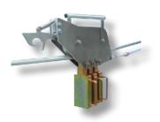
Recovering device to hook the robot in case of extreme inclination. Towing system by rope with detachable counterweights. Aluminium frame and wheels mounted on ball bearings and galvanised steel counterweights.
