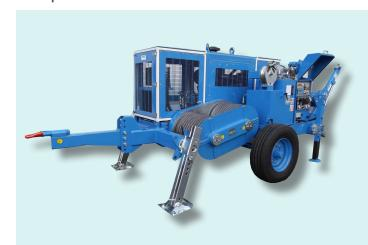
Hydraulic puller fit to pull one rope in stringing operations of overhead transmission lines. One hydraulic circuit allows to continuously vary the speed in both directions by operating one control device.
