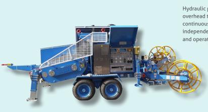
Hydraulic puller fit to pull one or two ropes in stringing operations of overhead transmission lines. Two hydraulic circuits allow to continuously vary the speed in both directions by operating two independent control devices. The two circuits may also be matched and operated together by one control device.
