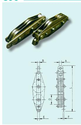
Tackle block for high voltage lines. Steel frame with 4 or 6 steel sheaves mounted on waterproofed ball bearings. Supplied in pairs.
