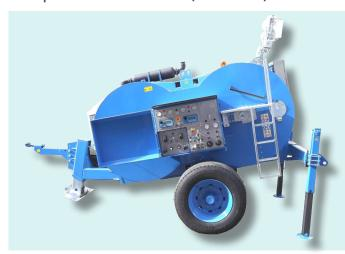
Hydraulic machine designed to operate both as a tensioner and as puller, fit to string one or two ropes or conductors.
