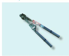
Ratchet cutters fit for conductors, cables and shield wires. The chain ratchet allows to cut the wire progressively with minimum effort. Insulated handles tested at 20.000 V.
