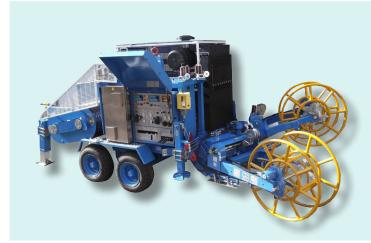
Hydraulic puller fit to pull one or two ropes in stringing operations of overhead transmission lines. Two hydraulic circuits allow to continuously vary the speed in both directions by operating two independent control devices. The two circuits may also be matched and operated together by one control device.
