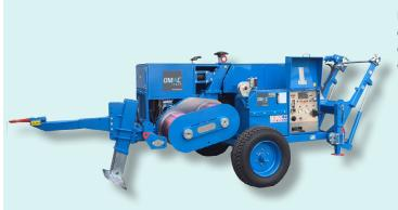
Hydraulic puller fit to pull one rope in stringing operations of overhead transmission lines. One hydraulic circuit allows to continuously vary the speed in both directions by operating one control device.
