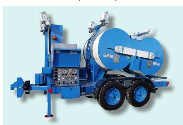
Hydraulic tensioner fit to string 1, 2, 3 or 4 conductors. Two hydraulic circuits allow to tension at constant force even varying the speed of stringing. The two circuits can be used independently or simultaneously, with automatic forces partition. Equipped with engine for pull-back performances. In pull-back mode, two hydraulic circuit allow to vary the speed in both directions, allowing to use one of the hydraulic circuits or both them matched.
