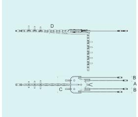
**Balanced type** running board for 4-bundle conductors fit for connecting the pulling rope to 4 conductors.
