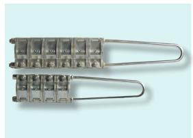
Multi-unit come-along clamp fit for pulling and anchoring overhead conductors and steel wire ropes. Made of steel elements, with aluminium liners for conductors. On request: bronze liners for wire ropes.
