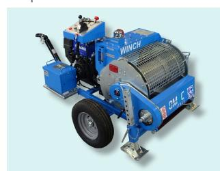
Hydraulic winch fit to pull one rope in service operations such as setting-ups and adjustment of transmission lines and underground cables laying. Direct pull on the drum. One closed hydraulic circuit allows to continuously vary the speed in both directions by operating one control device.
