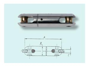
Swivel joint for ropes and conductors. Designed to release the torsion efforts during the pulling operations. Made of galvanised steel, complete with an axial bearing for an easy rotation.
