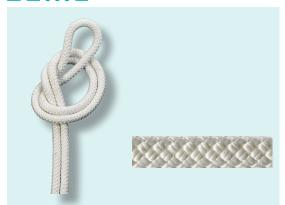
Pilot rope made of an external polyester mesh stocking and a hi-tenacity nylon core. Double torsion. Highly resistant to wear and UV rays. white colour. Supplied wound up on wooden reels or in coils.
