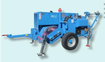
Hydraulic puller fit to pull one rope in stringing operations of overhead transmission lines. One hydraulic circuit allows to continuously vary the speed in both directions by operating one control device.
