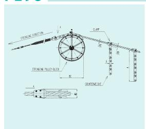
Antitwisting counterweight fit for stringing overhead fiber optics cables (OPGW). The counterweight allows to avoid the cable twisting during the passage in the running out blocks. Its shape is designed for passing in the grooves of the running out blocks without damaging the cable. A pair of nylon liners prevent damages to the conductor. Supplied in metallic case.
