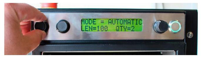
12 The next dial is used the adjust the length of the cushion - rotate right to create a longer cushion and rotate left for a shorter cushion. The minimum cushion length is 25cm and the maximum cushion is 5m
