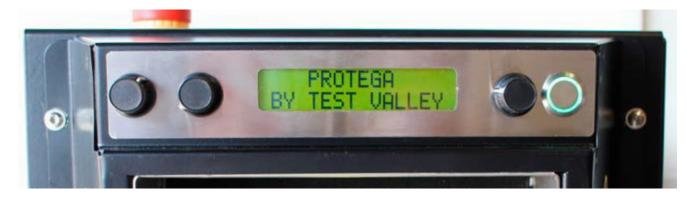
The first selection to make is to choose the mode you want to operate. Turn the first dial to the left to select 'On Demand' mode which will produce another cushion every time you remove one from the chute. Alternatively turn the dial to the right to select 'Automatic' mode which will produce a number of cushions every time you press the start button
