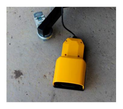
16 The foot pedal is connected to the machine as shown. The operate, press the pedal down until you have the desired cushion length and then release. The machine will cut the paper cushion once the pedal is released.
