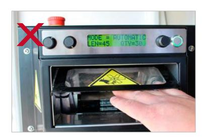
Liting the output flap will stop the operation of the machine. To reset, turn off the machine and restart.
