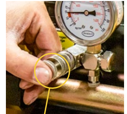
Push indent knob in to check pressure. (Nitrogen valve on post driver is similar to a tire valve.)
