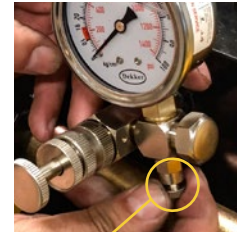
Make sure that the bleeder valve is closed.
