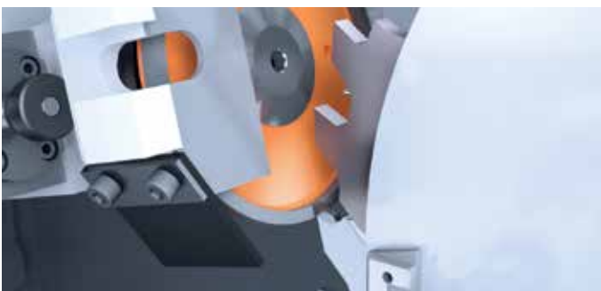
/// TOOTH TOP MACHINING on chipper segment from the saw mill industry
