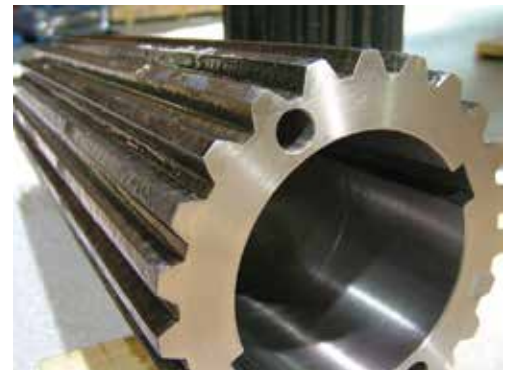
Dual-key, Involute-spline arbor sleeves
