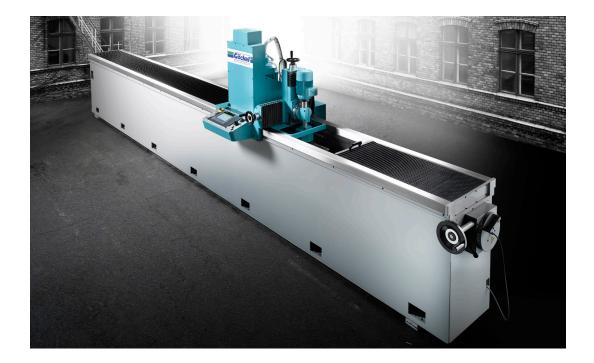
The Göckel G56ELT offers the highest quality grinding and control for improving veneer and OSB knife quality.
