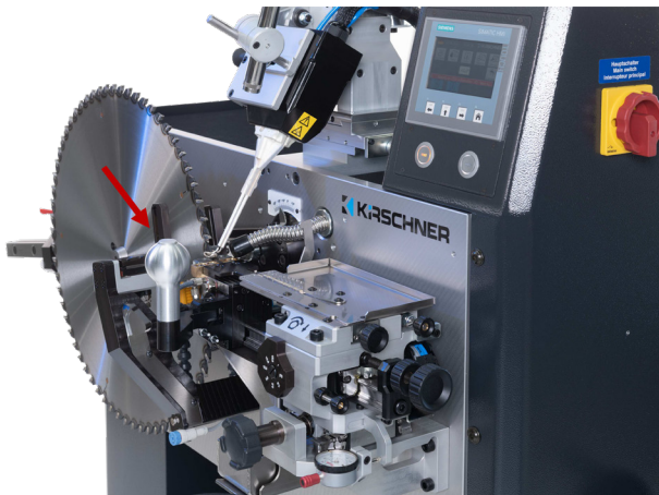
Process sequence, tip clamped centrally; easiest operation with the multifunction button
