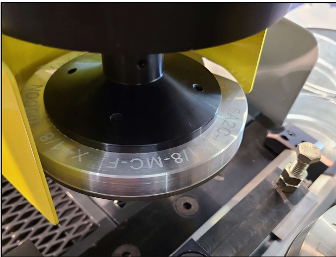
Auto Load uses 6" diameter diamond abrasive wheels
