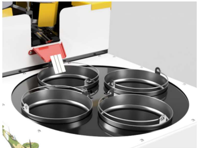
The Auto Honer measures each knife and automatically sorts based on quantity of cycles performed
