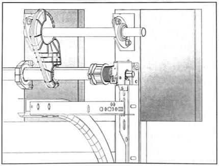
1. Prepare the mounting surfaces for mounting this kit and the opener. Solid mounting material or garage framing that is flush with the door track mounting surface should be used.
