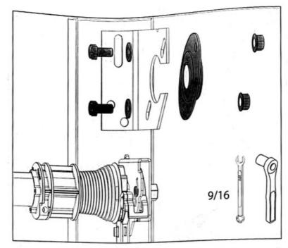
7. Loosely install oval bearing plates with bolts, washers and nuts provided on the right side of each bracket.
