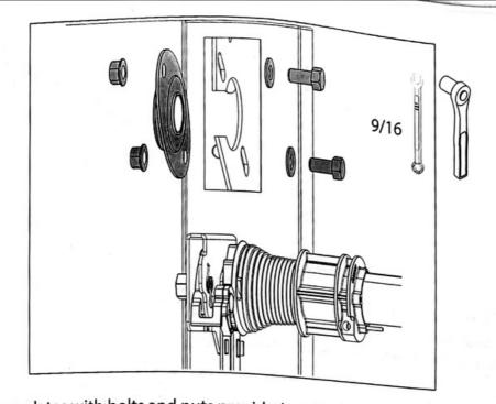
7. Loosely install bearing plates with bolts and nuts provided on the left side of each bracket
