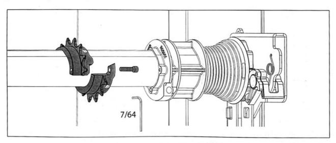
11. Install 2-piece sprocket onto TorqueMaster® shaft and assemble using a 7/64 in. allen wrench.
