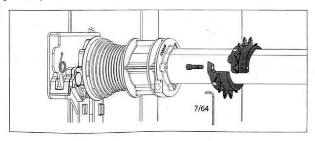
11. Install 2-piece drive sprocket onto TorqueMaster® shaft and assemble using a 7/64 in. allen wrench.
