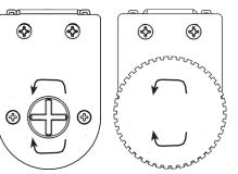
Turn counter clockwise to reduce spring tension.
