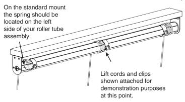
6B. **Front or Waterfall Mount:** Lift cords off the front of the roller tube assembly.
