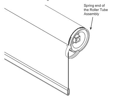
5A. The spring end of roller tube assembly should be rotating clockwise as you roll the fabric onto the roller.
