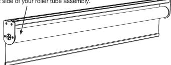
10. Lift the shade assembly up to the wall brackets. Hook the back side of the head rail onto the back side of the wall brackets. Then, rotate the shade assembly up until it snaps into each of the wall brackets.
