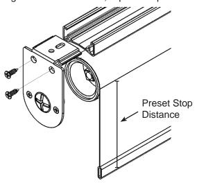
8. Attach the wall mounting brackets. Use a bracket at each end of the track between 1" and 3" from the end of the head rail. Then place brackets no more than 24" apart over the remainder of the track. Securely attach all brackets to the mounting surface.
