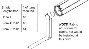
7. If you want the shade to stop at a set distance from the top, unroll the fabric to that preset distance before you install the end brackets. Slide the end brackets into the head rail and onto the tube assembly. Secure into place using the screws provided with the end brackets. (One side is shown...repeat for the other side). Be careful not to release the spring tension when installing the end bracket onto the spring end of the tube assembly. If the spring tension is released, repeat Step 6.
