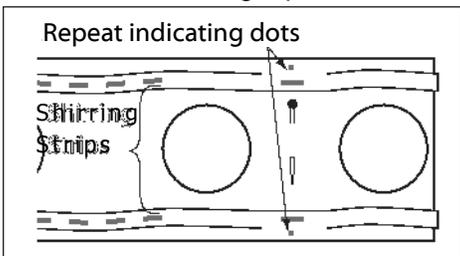
3. Lay the tape across the panel with shirring strips up, have the straight pin aligned with one edge of the panel. At the other edge of the panel, find another set of repeat indicating dots. Mark it with a straight pin also.
