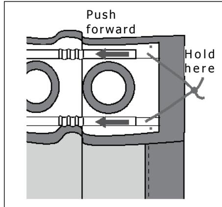
Do not cut off the excess cords. Wind the loose cords to make a neat bundle. Catch the cord bundle with two stitches to the panel.
