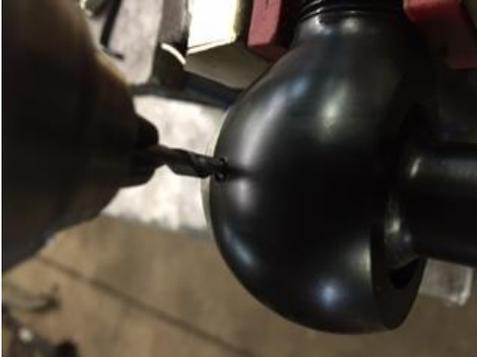
Step 5: Put the set screw back in and put a dab of purple or blue loctite on the screw to ensure it stays in place longer. Screw it in nice and tight using an allen key. This set screw is what holds the cap in place so it's important, even though it's small.
