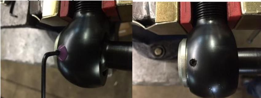
Step 16: Grease it up! Tie Rod Ends should take a couple pumps from a grease gun. You can then lap the pin again if you want to ensure grease is evenly distributed around the pin.
