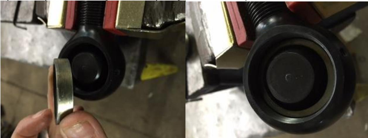
Step 11: Using your fingers, spread the spiral lock apart and insert the end of it into the groove in the body. Hold it there while you get the pick and press down on the end and slide the pick around the spiral lock so it will set into place. It should sit nicely inside the groove in the body.
