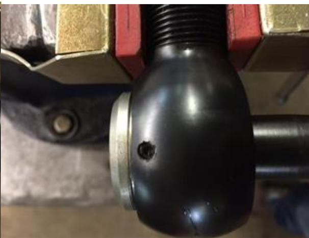
Step 16: Grease it up! Tie Rod Ends should take a couple pumps from a grease gun. You can then lap the pin again if you want to ensure grease is evenly distributed around the pin.
