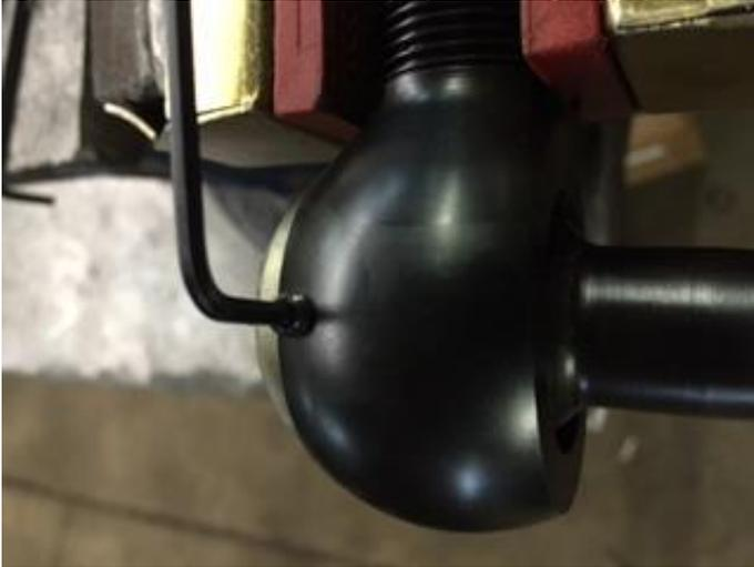
Step 3: Using a spanner wrench or a Pipe Wrench if you do not have a spanner, remove the back cap by unthreading it.
