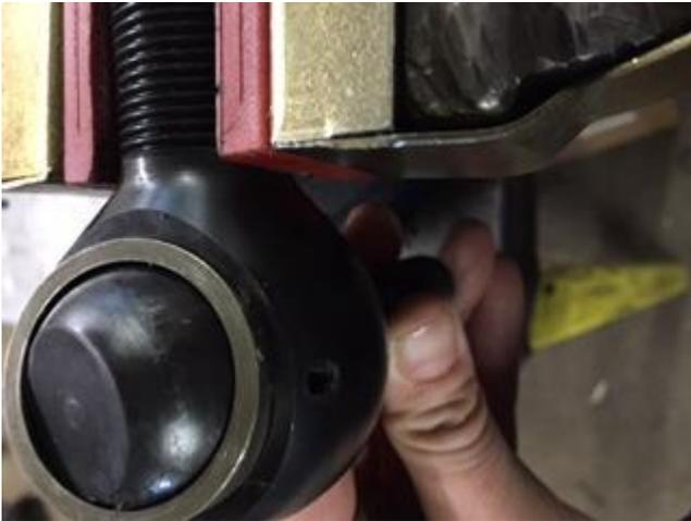
Step 6: The bottom race will still be inside. Use your fingers to wiggle it up and out of the body. If the races don't need to be replaced, you can leave it in there or take it out, clean it and put it back in.
