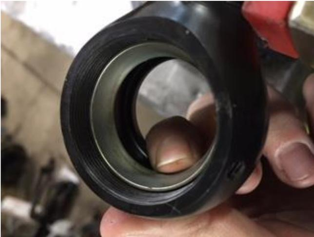
Step 7: You will notice there are 2 types of races. One with a Chamfered Edge and the other with a Square Edge. The Chamfered Edge race goes in first (bottom) and the square goes in on top after the pin.
