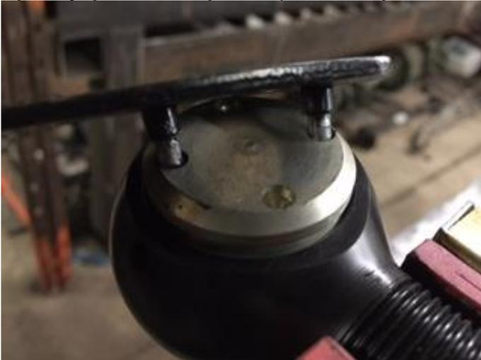
Step 4: Once the cap is off, you will see a spiral lock holding the inner races and pin inside. Take a pointy pick of some sort and find the end of the spiral lock. Then proceed to run the pick underneath and take the spiral lock out.
