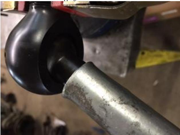
Step 14: Once you have it tightened, take a drill bit that fits inside the set screw hole (in most cases it is a #21 bit) and put it into your drill. Next you want to drill a small indent into the cap threads so the set screw can seat in place. Don't drill too deep – just enough to see an indent. \*\* This can be done over and over without any negative affect to the cap or threads \*\*
