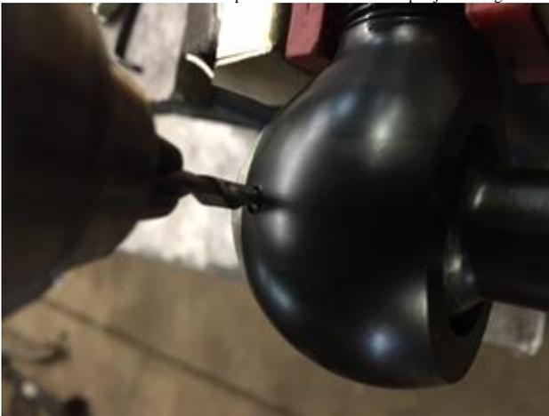
Step 15: Put the set screw back in and put a dab of purple or blue loctite on the screw to ensure it stays in place longer. Screw it in nice and tight using an allen key. This set screw is what holds the cap in place so it's important, even though it's small.
