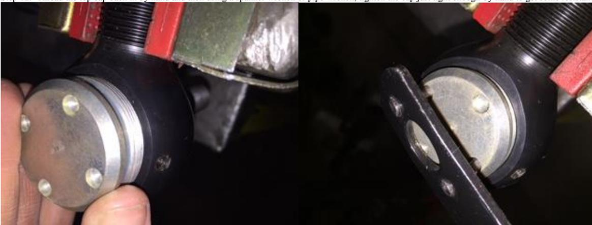
Step 13: Check the pin by placing a tube or something over the pin to lap it back and forth. It should feel firm – not too loose that it can be moved easily by hand, but not too tight that you can't move it at all with the lapping rod.
