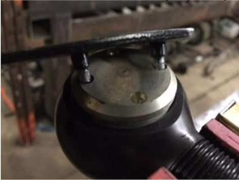
Step 4: Once you have it tightened, take a drill bit that fits inside the set screw hole (in most cases it is a #21 bit) and put it into your drill. Next you want to drill a small indent into the cap threads so the set screw can seat in place. Don't drill too deep – just enough to see an indent. \*\* This can be done over and over without any negative affect to the cap or threads \*\*
