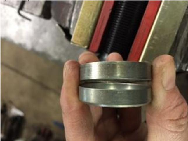
Step 8: Clean the inside of the body out with a rag to ensure no grease or grit is inside before you rebuild. Put the Chamfered Race into the body and press all the way down to the bottom with your fingers.
