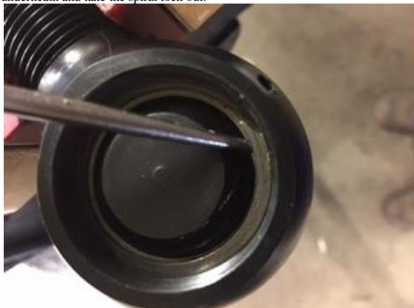
Step 5: Push up on the pin from the bottom to pop the top race and pin out of the body. If it is difficult to remove, take the joint out of the vise, turn the joint over and gently tap the body flat on a table until the top race comes out.
