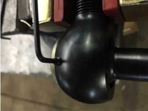
Step 3: Using a spanner wrench or a Pipe Wrench if you do not have a spanner, tighten the cap on the back as tight as you can go by hand – Do not go to the point where you risk breaking the spanner wrench, it doesn't need to be that tight... just enough to snug the pin up.
