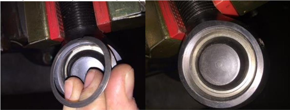
Step 12: Thread the top cap back in by hand and then using a spanner wrench or pipe wrench, tighten the cap just tight enough by hand to get some resistance.
