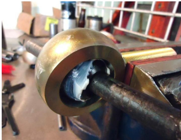
**STEP 9:** Once the ring is set, drill into the ring through the set screw hole using a #21 bit or a 7/32 (depending on the set screw size) Warning hold the lock ring with the spanner wrench of the ring will spin loose as you're drilling.
