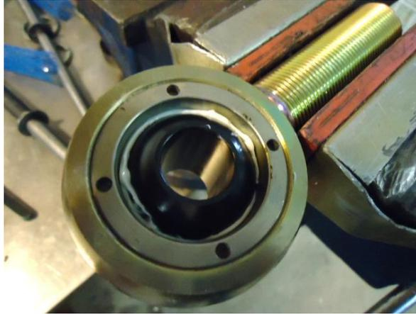
**STEP 8:** Insert a piece of steel, a screwdriver or anything you have into the through-hole to lap the ball and make sure it is set correctly. You should be able to lap it back and forth with a little tension but it should still move freely with no binding, grinding or any sticky spots. If you can't move the ball, you tightened the ring too much.
