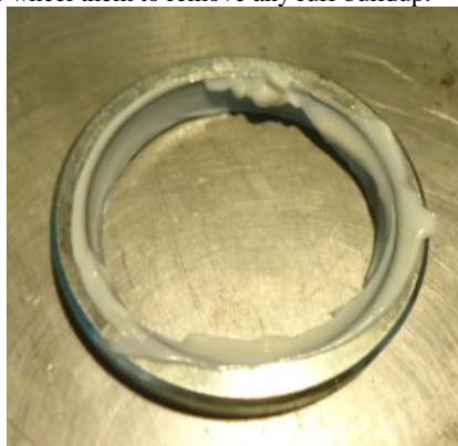
**STEP 3:** Line the inside of the cup with grease.
