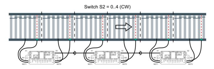
If the conveying direction is reversed, only the direction setting on switch S2 has to be changed, the cabling remains the same. The direction setting defines, which of X1 and X2 the downstream and upstream connector is.
