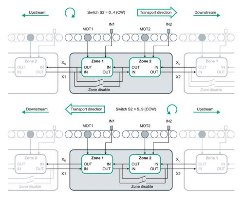
The Motor Control Module contrains two of those zone controllers, which are connected internally to form a chain of two zones. Each of the **MOT, IN, X** connectors are directly connected with the respective zone controller.
