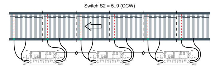
Note: The Motor Control Modules never require you to build cable loops like in the following image. Building such loops will bring the connected zones into wrong logical order, which will prevent correct operation.
