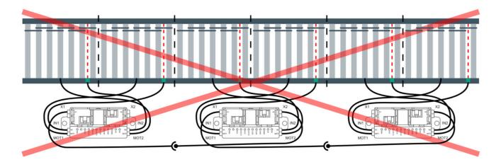
If the Motor Control Module should control a single zone, the corresponding motor and photo eye are connected to the downstream side of the module. In single zone mode the upstream side motor is synchronized with the other one, so it can be used to support the other motor (e.g. for heavy loads or climbs).
