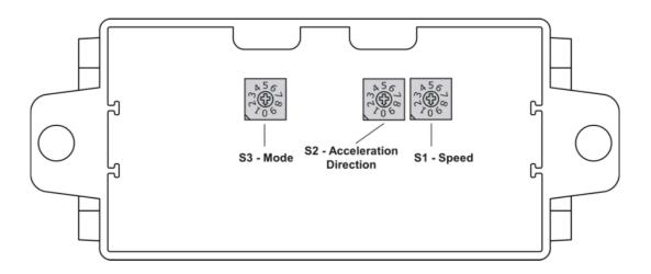
Note: The configuration of the switches is applied at power up. To change the configuration the Motor Control Module has to be repowered after modifying the switches. Motor power supply fuses are not replaceable.
