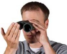
**2. Adjust the diopter**—start by closing your left eye or covering the left objective lens with your hand. Lift the diopter ring to unlock and, looking through your right eye, adjust the diopter so that the object is in focus. Make note of this diopter setting in case you need to set it again. Push the diopter ring down to
