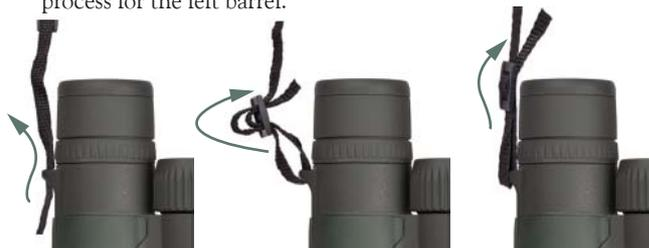
1. Push a few inches of the strap through the strap attachment on the binocular.
