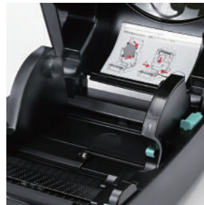
Drop-in label roll holder for easy media installation
