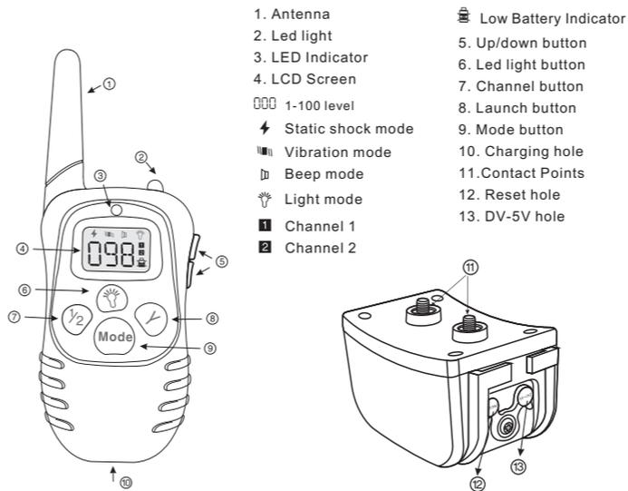
1. **Antenna:** Transmits the signal from the Transmitter to the Receiver Collar.
