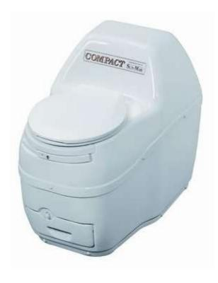
The Sun-Mar Compact separates liquids from solids after they enter the main composting chamber by using a patented bio-drum feature. Solids are passed onto a finishing drawer once broken down and liquids are evaporated away by a heating tray and air movement caused by an internal vent fan.
