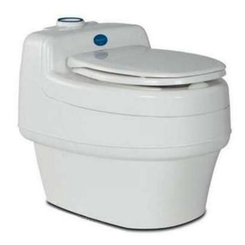
The Villa compost toilet was designed to look and feel as close to a traditional toilet as possible to make it easier for new users to adapt to using it. It can be used with on-grid use, as well as AC/DC configurations for those who want to run it in a 12v environment. You will have to install a vent pipe for the removal of odors outside of the building.
