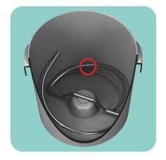
The **agitator bar** spins for 2 minutes while mixing after a solids use.
