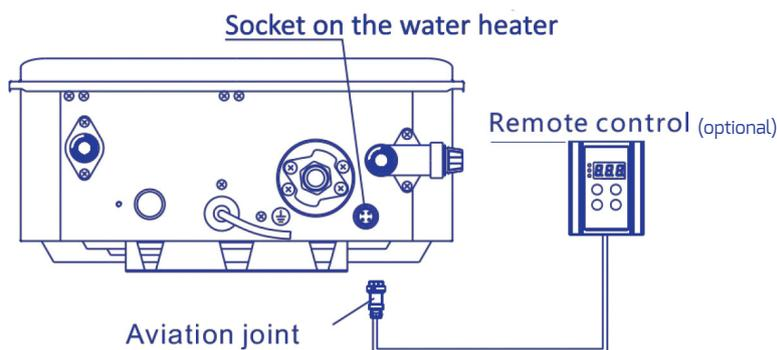
2. For two controls: First, cut off the aviation joints on the two controllers, plug one into the socket on the water heater (length is dependent on your requirements), and throw away the other. Then connect the wires of the aviation joint to the inlet wire of the connector, and connect the two remote control to the outlet wires of connector.
