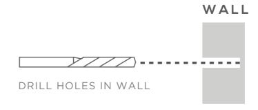
TIP: Blow dirt out of hole. WALL
