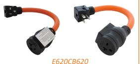
This AC WORKS® brand protective extender is heavy-duty. This 1-foot cord is a NEMA 6-20P to NEMA 6-15/20R. The NEMA 6-20P is a 20 Amp, 3-prong, straight-blade plug. The NEMA 6-15/20R is a 15/20 A, T-blade, 250 Volt female connector. The cable is an STW, 12/3, anti-cold weather cable that stays flexible in extreme temperatures. The cord is super durable and typically used with construction and/or industrial equipment.
