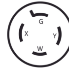
NEMA L14-20P NEMA L14-20R 20 Amps 125/250 Volts Commonly used in industrial locations and generators.
