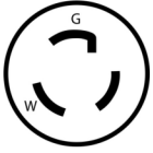
NEMA L5-15P NEMA L5-15R 15 Amps 125 Volts Commonly used in industrial locations.
