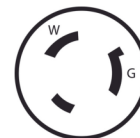
NEMA L7-20P NEMA L7-20R 20 Amps 277 Volts Commonly used in industrial locations.
