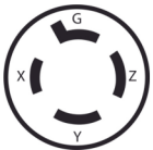
NEMA L15-20P NEMA L15-20R 20 Amps 250 Volts Commonly used in industrial locations.
