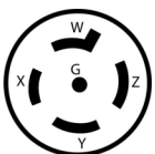
NEMA L22-20P NEMA L22-20R 20 Amps 277/480 Volts Commonly used in industrial and warehouse locations.
