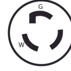
NEMA L7-15P NEMA L7-15R 15 Amps 277 Volts Commonly used in industrial locations.
