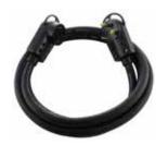
L1430M50 - The cord comes in 10, 25, 50, 75, and 100 feet in length. It is a NEMA L14-30P to NEMA SS2-50R. The L14-30P is a 30 Amp, 125/250 Volt, 4-prong male locking plug. The SS2-50R is a 50 Amp, 125/250 Volt, 4-wire female. It features an STW 10/4, 600 Volt jacket, 30 Amp Copper wires, and has an anti cold weather rubber cord staying flexible in extreme temperatures. (Continued on Page Two)
