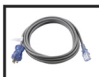
MD170-AL PLUG: NEMA 5-15P CONNECTOR: IEC LOCKING C13 RATING: 13 AMP 125 VOLT CORD: SITW 16/3 LENGTH: 10 FEET
