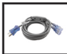
MD115-Y PLUG: NEMA 5-15P CONNECTOR: (2) IEC C13 RATING: 10 AMP 125 VOLT CORD: SITW 18/3 LENGTH: 10 FEET
