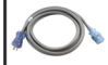
MD261-AL PLUG: NEMA 5-15P CONNECTOR: IEC LOCKING C13 RATING: 15 AMP 125 VOLT CORD: SITW 14/3 LENGTH: 15 FEET
