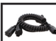
CC14Y515 PLUG: IEC C14 CONNECTOR: (2) NEMA 5-15R RATING: 10A 125V CORD: SITW 18/3 LENGTH: 7 FEET
