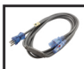
MD171-ALY PLUG: NEMA 5-15P CONNECTOR: TWO LOCKING C13 RATING: 13 AMP 125 VOLT CORD: SITW 16/3 LENGTH: 10 FEET
