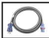
MD173-AL PLUG: NEMA 5-15P CONNECTOR: IEC LOCKING C13 RATING: 13 AMP 125 VOLT CORD: SITW 16/3 LENGTH: 15 FEET
