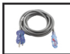
MD115-AL PLUG: NEMA 5-15P CONNECTOR: IEC LOCKING C13 RATING: 10 AMP 125 VOLT CORD: SITW 18/3 LENGTH: 10 FEET
