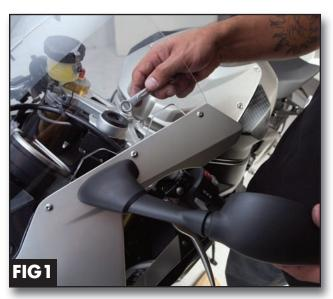
**Fig 1.** Remove both mirrors. The fasteners are behind the fairing. Be careful not to drop the mirrors!
