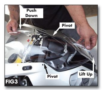
**Fig 3.** HERE IS THE TRICKY PART! You have to carefully recline the windscreen down from the fairing. It will be pivoting in two places one on each side. (See FIG3A).
