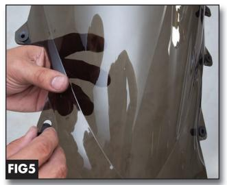
**Fig 5.** Before installing Zero Gravity Windscreen. Install Rubber wellnuts (Remove them from your stock screen).
