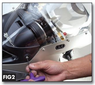
Fig 2. Remove all 8 fastener screws.
