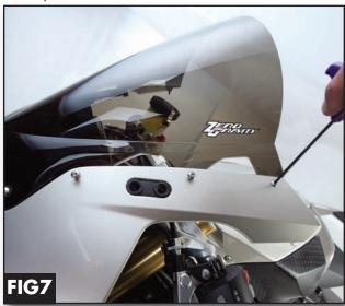
**Fig 7.** Starting from the top of the windscreen and working down, hand tighten all fasteners then reinstall mirrors.
