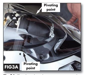
**Fig 3A.** This photo shows he pivoting points on either side of the screen. **Be careful not to over pivot!**
