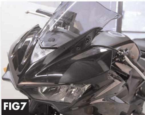
**Fig 7.** At this point the fairing is mostly loose, and is only held in place by several clips. To remove, standing in front of the bike and pull it evenly and firmly straight towards you (as shown in the video).
