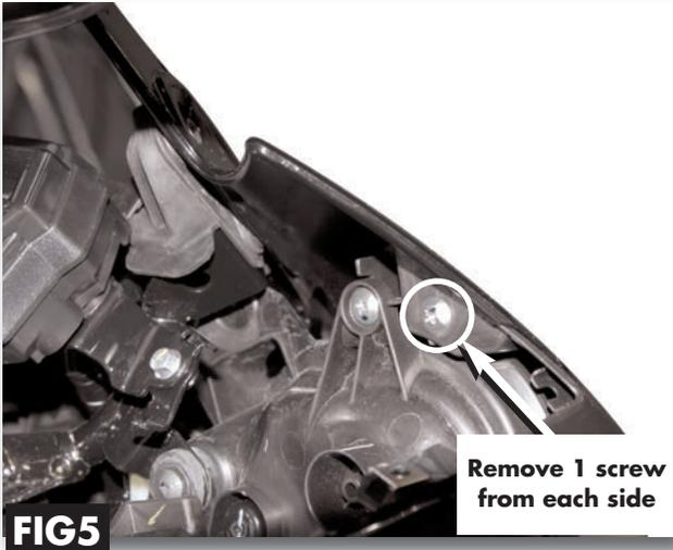
**Fig 5.** Remove the two screws on either side of the headlight housing that fasten the front fairing to the headlight.
