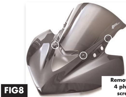
**Fig 8.** Remove the four plastic phillips screws that hold the windscreen in place.
