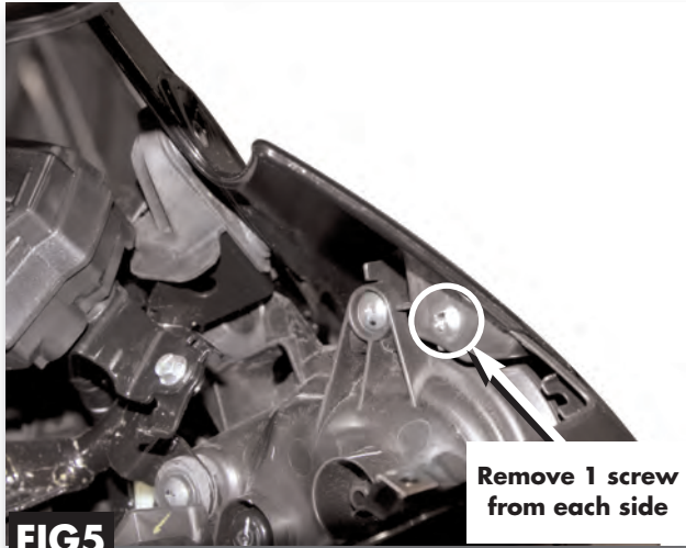
Fig 5. Remove the two screws on either side of the headlight housing that fasten the front fairing to the headlight.
