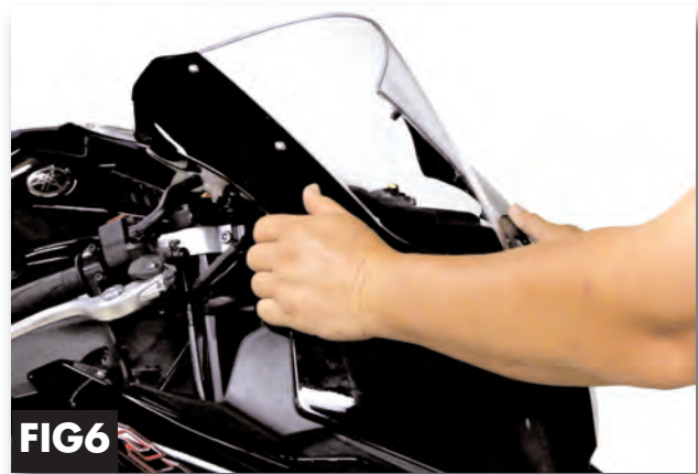
Fig 6. To remove, stand in front of the bike and pull it evenly and firmly straight towards you (as shown in the video). To visually see this, we made a YouTube video. Scan this QR code with your mobile phone, it will take you straight to the video or click below for a quick video.
