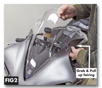
Fig 2. Start by inserting the windscreen from one side. To slide in, grab and pull up on the upper fairing as shown above. Rotate the mirror rubber gasket to align the side windscreen humps. Repeat for the other side. For 2012 - 2014 install Tip: The trick to keeping the two plastic units together, is to not flex the windscreen during the process.
