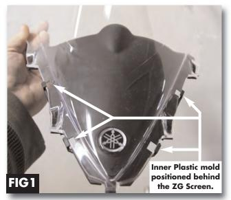
Fig 1. Remove both mirrors. Locate both fasteners in the inside fairing. Once you remove the mirrors the factory screen can be removed by sliding back and pulled up slightly. For 2012 - 2014 install: OEM windscreens have an inner plastic mold attached to the screen (as shown above). Carefully remove it and attach to Zero Gravity screen as shown in Fig 1.
