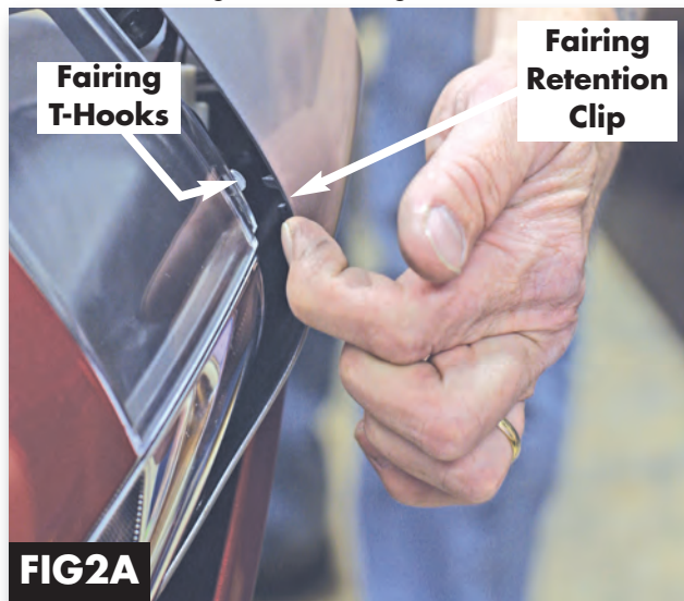
Fig 2A. HERE IS THE TRICKY PART! Locate the fairing retention clip and windscreen T-Hooks before applying any movement pressure . There will be two T-Hooks, one on each side. (See FIG3 ).
