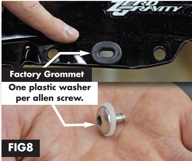
FIG 8. Remove both left and right factory rubber grommet and install them to Zero Gravity screen (as shown above.) Then assemble one small plastic washer (provided) to each of the four factory allen screws.
