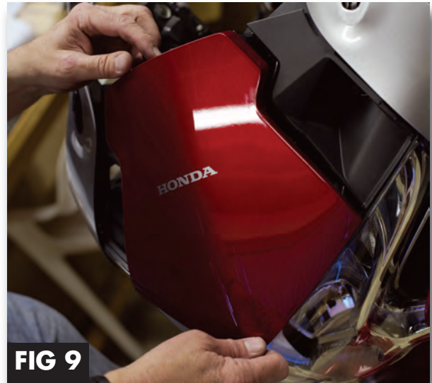
Fig 9. Replace finish plate back to it's respected location. Starting from the bottom clip and work your way up.
