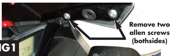
Fig 1. Remove both mirrors. Locate both fasteners located on the inside fairing. Also, remove inner plastic that's covering both left & right two allen screws.
