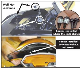
**Note:** If the two upper fasteners are not grabbing the wellnut threads, you will have to reach behind the two upper wellnuts and push them against the fasteners to start the screwing process.
