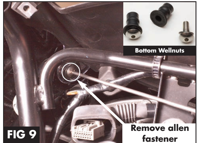
Fig 9. Remove 2 allen fastener at the bottom windscreen, viewing from the inside fairing. (For Both Sides) See FIG9.
