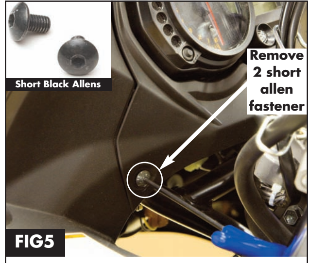
FIG5 Remove 2 short allen fastener Fig 5. On the same plastic fairing, remove 2 black short allen fastener located on the bottom of the instrument cluster. (For Both Sides) See FIG5. Note: The finish allen screws are in Black.
