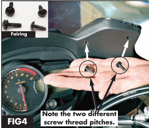
FIG4 Note the two different screw thread pitches. Fig 4. Looking from the upper inside fairing. Remove total of 4 screws, and take note of the different thread pitches. (For Both Sides)
