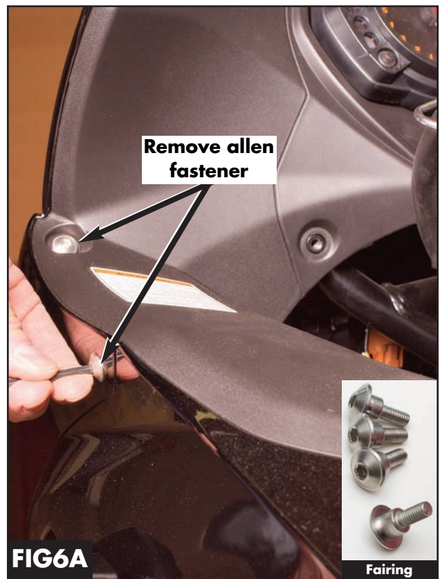
Remove allen fastener FIG6A Fig 6A. On the same plastic fairing, there are 4 silver allen fastener located on the top and the sides. (For Both Sides) Note: The finish allen screws are in Silver.
