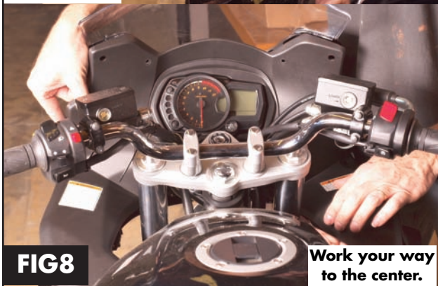
Fig 8. Now you are ready to separate the inner fairing from the bike. Start from the two tail ends and start dislodging and working your way to the inside.
