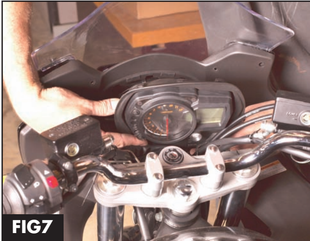
Fig 7. Remove instrument panel by pulling it apart from the fairing frame. The wire harness needs to be disconnected before fully removing. USE CAUTION TO NOT OVER PULL!!!
