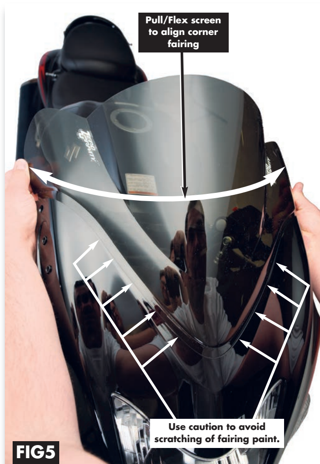
Fig 5. After inserting the middle screen tab into fairing, use both hands to lightly bow the windscreen and carefully insert into the inside fairing. Massage the screen to place into the fairing.
