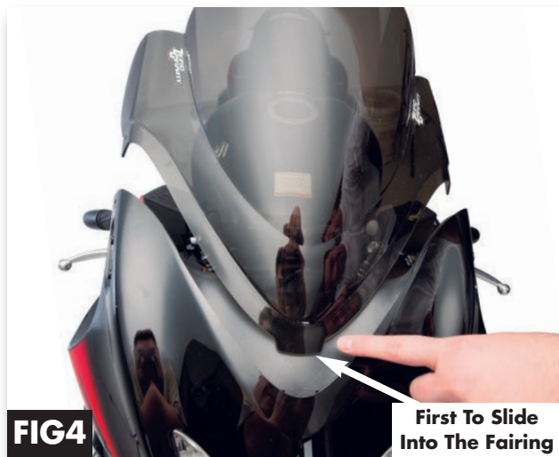
Fig 4. After removing the stock screen, the Zero Gravity replacement is installed/removed just like the stock screen. The tab in the front of the screen is the first to slide into the fairing.
