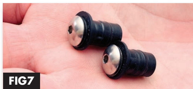
Fig 7. Now you are ready to lock the screen into position. Locate the two Allen screws and Wellnut removed from the dismantled stock screen. Put them together like this, slightly screw the Allens into the wellnuts.
