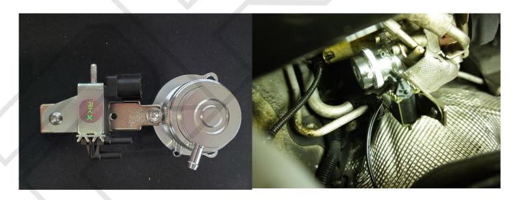
3. Install the new wire harness by connecting one end into the solenoid and the other into the original diverter valve connector.
