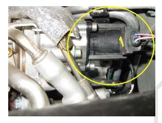
2. Secure the new diverter valve in place with the top two bolts. Attach the solenoid to the mounting bracket using the supplied Allen head bolt. Secure the bracket to the diverter valve using the third bottom bolt.
