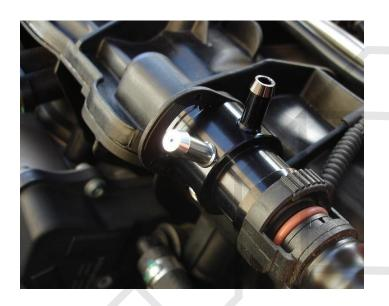
5. Route vacuum hoses as shown. Use a silicone lubricant to ease the instillation of the hoses as fitment is tight! Use zip ties on all vacuum hose connections. Route the vacuum lines away from the exhaust and moving parts.
