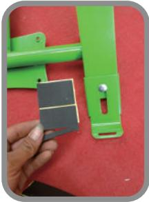
**8** Stick the protection pads on the bottom of the SkyKart.
