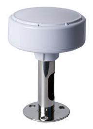
SA-200 is the integration of the high performance GPS patch antenna and a state-of-the-art low noise amplifier into an extremely compact/fully waterproof enclosure and when connected to a GPS receiver with +5VDC antenna power it can provide excellent antenna signal amplification and out-band filtering with rejection for that receiver.
