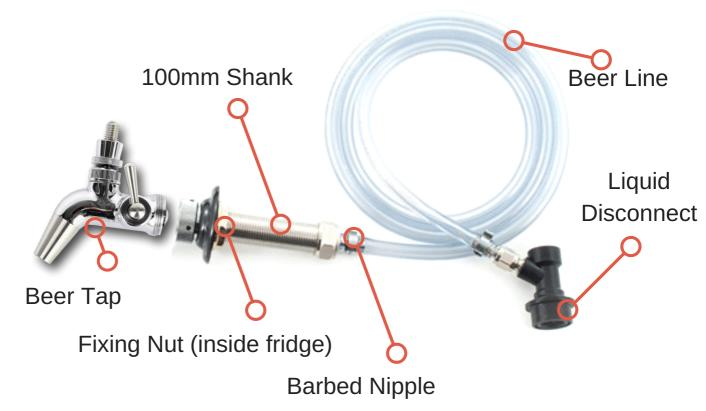
For using with eskies or fridges this allows you to attach the taps externally. All you need to do is drill a 22mm hole through the surface.
