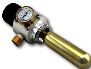
Professional CO2 Mini Regulator. NOTE - Always check reg is OFF then screw in CO2 Bulb quickly until hiss stops. Serving Pressure approx 3-4PSI. Storing Pressure approx 10-12PSI. Force Carbonating Pressure 20-25PSI.
