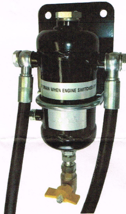
Fully assembled FGV-2 with swaged fittings
