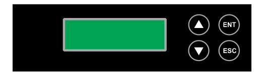
Control Buttons: There are 4 control buttons: ▲ ▼ ENT ESC
