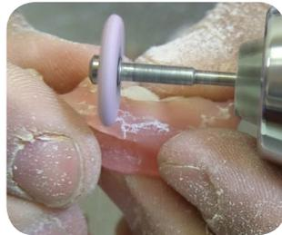
**2.** Round the edges of the TCS Pink Grinding Wheels with a truing stone. Use these wheels for major reduction and to begin creating anatomy. Use continuous movement, high speed with moderate pressure.
