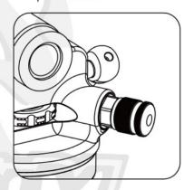
**Negative air chamber** Supply air pressure according to pressure meter
