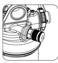
Compression Adjuster + direction rotation, lock-out - direction rotation, open up
