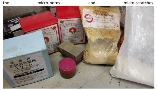
After 8 'layers' the lacquer was polished with migako powder. First a mixture of migako powder and rapeseed oil is rubbed over the surface with your finger tips and cleaned off. Then then the same is done with dry migako powder.
