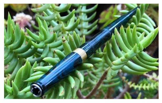
Before starting with the urushi process, I wet sanded the holder with a 1000P sanding paper, mainly to get off any residual oil that was used during turning or polishing.
