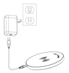
Connect a USB wall charger to the wireless charging Pad When the charger is correctly connected to the wireless charging Pad the indicator light flashes blue, green and cyan then turns off.
