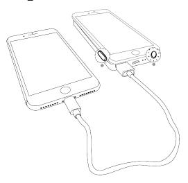
Connect the cable and tap the side button to charge the mobile device.
