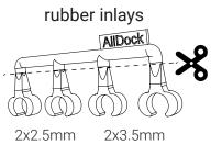
The rubber inlays are provided for the adjustment of the height of the connector to the respective mobile phone protective cover. The thicker the protective cover, the larger the inlays that need to be used.
