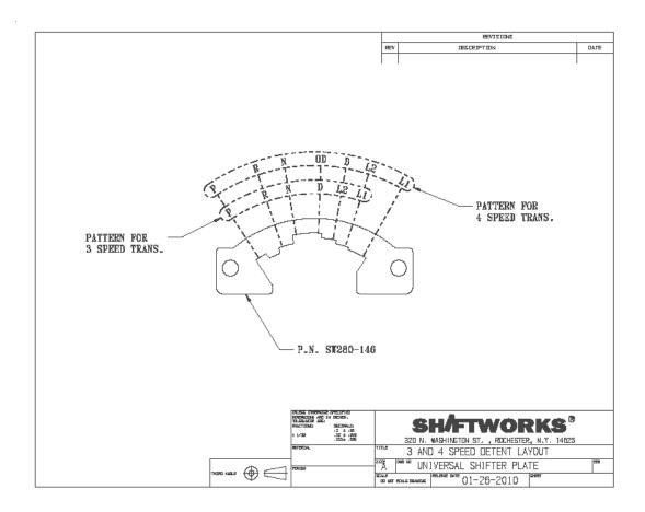
Your Shifter will work for BOTH the 3-speed & 4-speed OverDrive transmissions.
