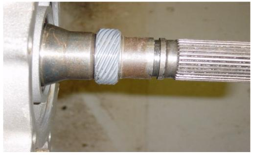
Install o-ring into groove of tail housing.
