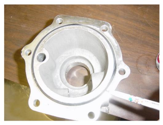
Install tail housing onto transmission body using your existing six bolts.
